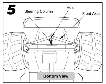
• Fit the curved end of the steering column into the hole in the front axle.
